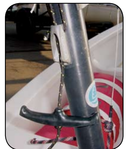
Handle tied to the sprit line will help you to adjust the sprit when sailing.
