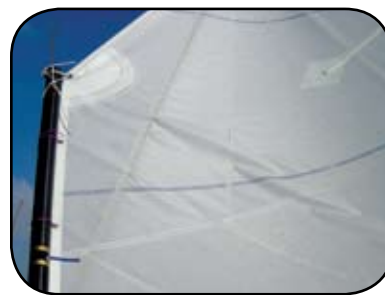
Right sprit tension. A little wrinkle perpendicular to the sprit is ok.
