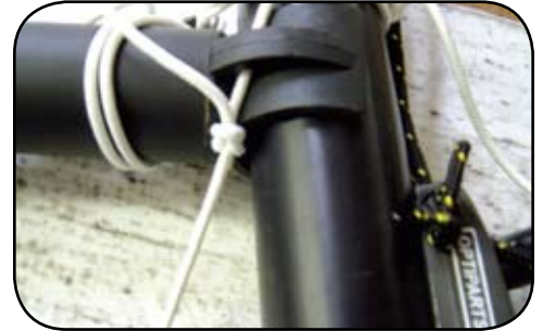
A square knot to help adjusting the preventer.
