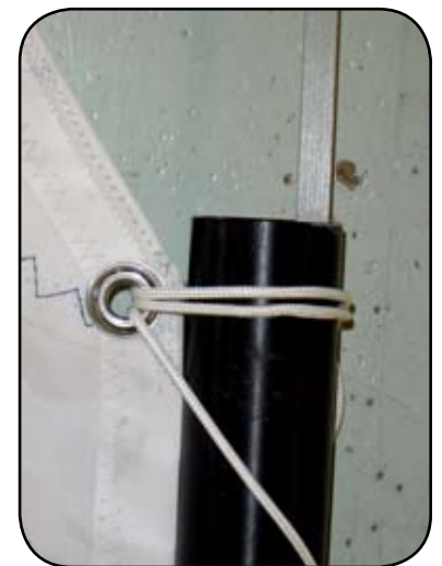
Tying the preventer. Not any looser than that
