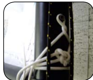
Tightening the preventer for light air - two twists
