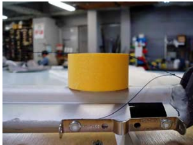
Diagrams 1 & 2: Use a roll of tape to support tensioned string at measurement points
